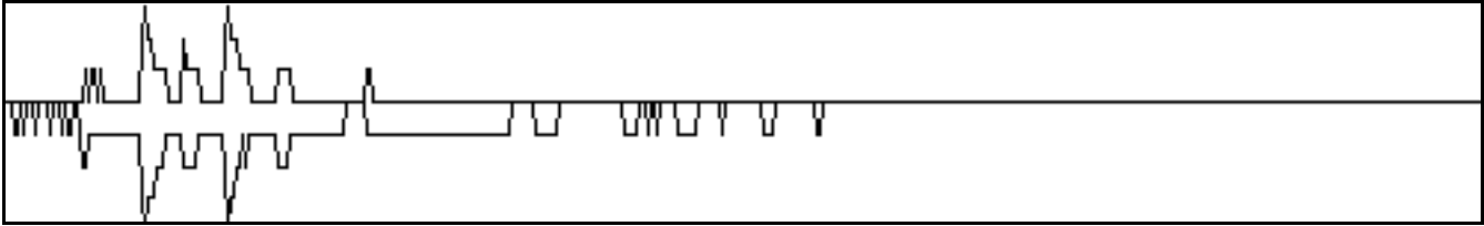
Figure 7: Piano with truncation. Note that the last few notes are well below the least significant bit.
