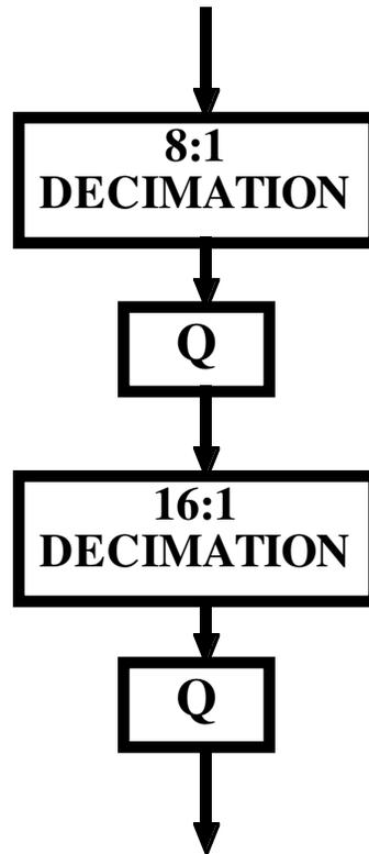
**Figure 2: A diagram of a 2-stage 128:1 decimation filter. We have inserted a block labeled “Q” to make explicit the undithered quantization that necessarily follows each stage. We hypothesize that these quantization blocks contribute to the audible differences. This would suggest that the fewer decimation/quantization stages that are present, the higher the audible quality.**
