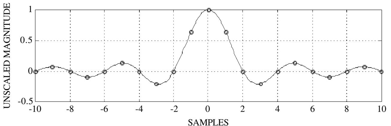
**Figure 3: Time-domain representation of a possible decimation filter for use in an oversampling converter. Note that a maximum occurs at 5 samples removed from the center, which corresponds to a delay of 50 microseconds in this example.**
