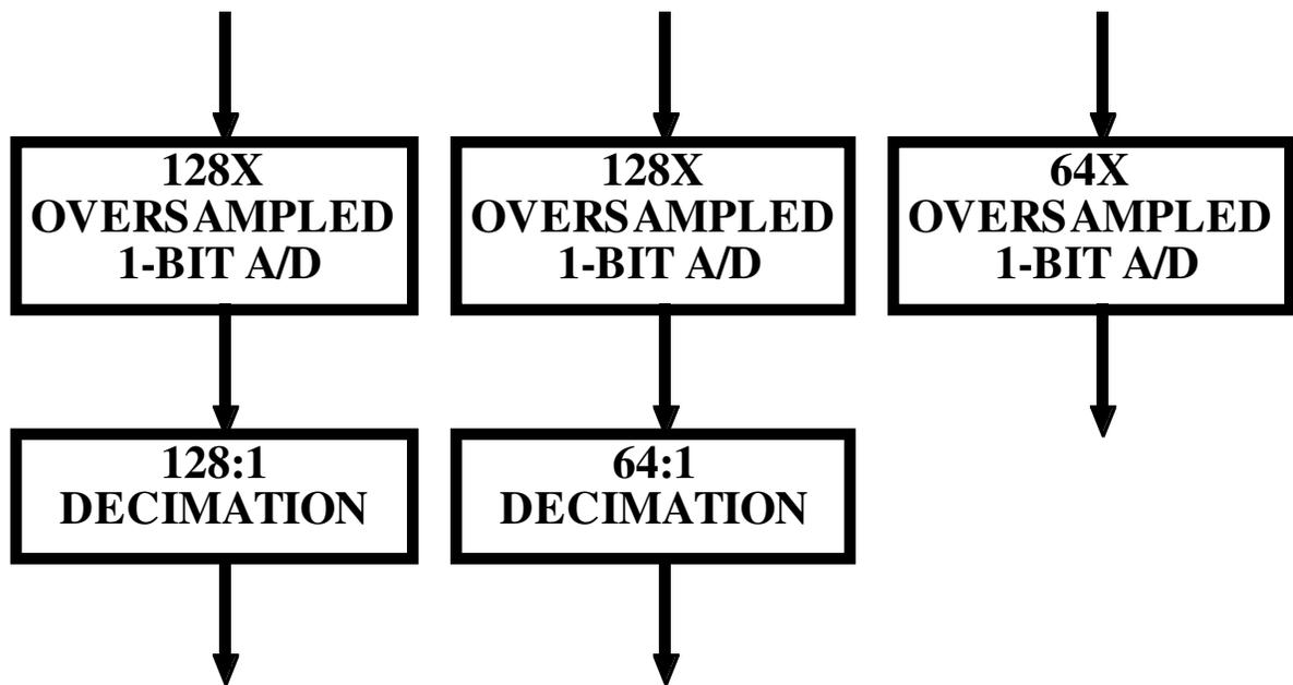
**Figure 1: Comparison of the conversion chain for a 44.1 kHz converter, an 88.2 kHz converter, and a DSD converter. The key point is that the higher sampling rate converters generally involve fewer stages of decimation.**
